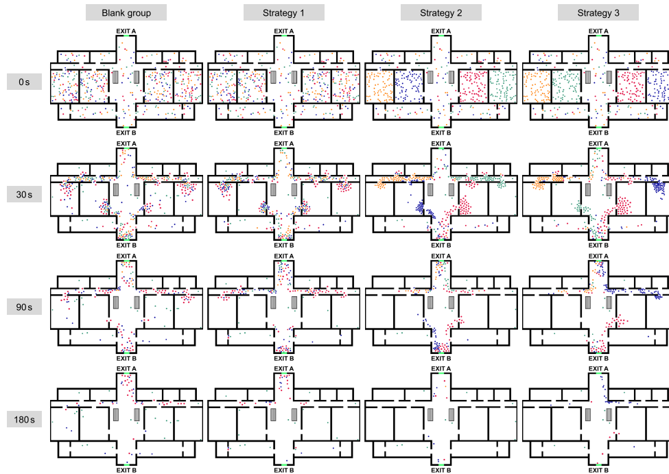
Fig. 11. Snapshots of mixed crowd evacuation in the library scene under different management strategies. The vertical direction indicates different moments at 0, 30, 90, and 180 s. The horizontal direction denotes different management strategies. The orange, blue, green, and pink circles represent nondisabled, visual-disabled, acoustic-disabled, and physical-disabled pedestrians, respectively.
